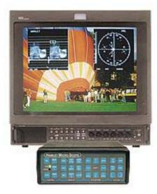
Weighing in at only 655gram (23 oz) this composite waveform/vectorscope with audio monitoring is extremely versatile. With a full range of time base functionality, including Hands Free Timing, trace display options, it's powered by in-built re-chargeable batteries or via its 12Vdc adapter (included). Available as NTSC or PAL options include an SD SDI input\* and Protective Carry Case\*.
