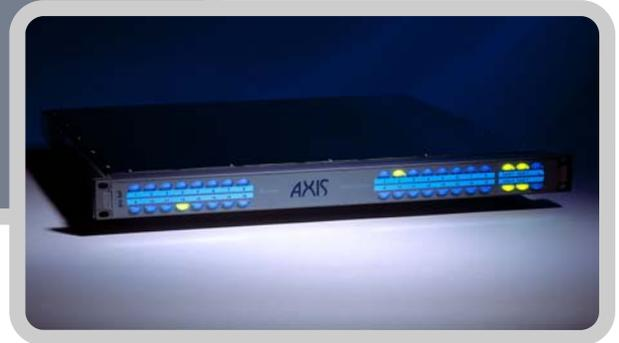
Axis is a compact range of 16 x 16, 1RU self-contained routing switchers that addresses a wide range of audio visual routing requirements from traditional broadcast to new mediacasting technologies.
