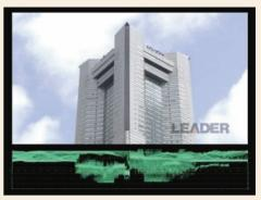
Picture and waveform time axis correspondence
