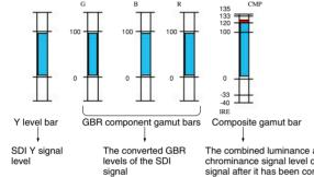
The combined luminance and chrominance signal level of the SDI signal after it has been converted to a composite signal.
