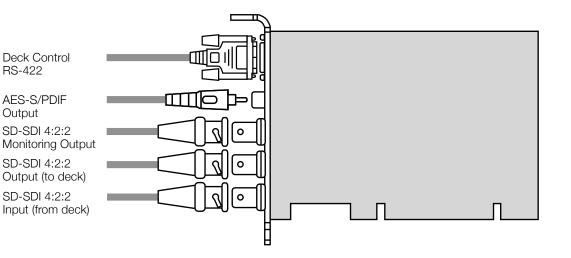
This DeckLink model does not have genlock, so you need to connect your deck to the Deck SDI Output, which has stable output to sync the deck. Set the deck to input or auto reference. Be sure to set the "Black Video Output to Deck in Capture" option to "On Digital SDI Outputs" in the DeckLink control panel, when using this feature.
