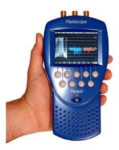
The Hamlet Flexiscope is a multi-format multistandard handheld waveform, vector, audio, picture monitor. Using a built-in 3.5" diagonal high quality TFT display shows the picture in 4:3 or 16:9 formats. Also shows conventional waveform, vector and audio displays together with data analysis.
