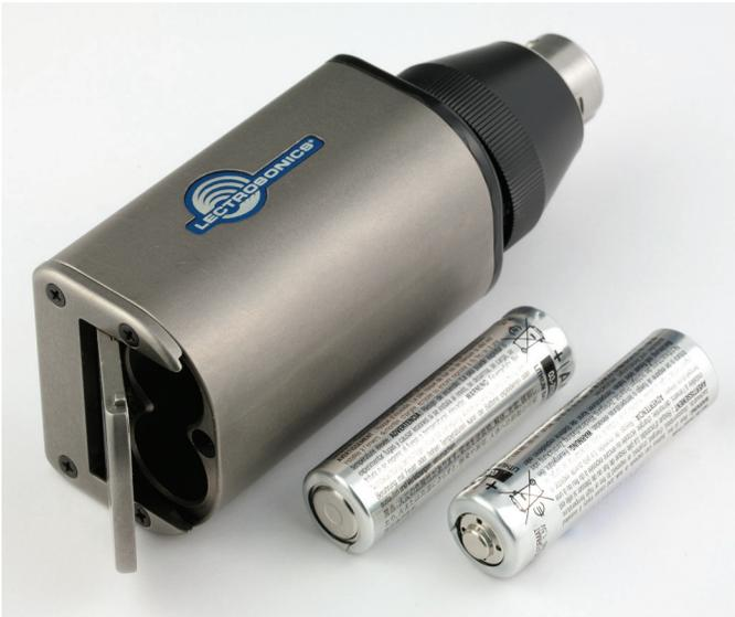
The battery compartment door is hinged to the housing and remains attached to the transmitter when opened. It securely latches in place and applies pressure to the batteries when closed. The two AA batteries are connected in series through a conductive plate on the door.
