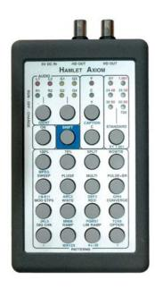
The Hamlet Protean Axiom is a small high definition SDI video and audio generator. Using leading edge technology Hamlet has produced a compact, low power; hand held, HD SDI video and embedded audio generator, 13 standards, and 16 fully compliant SMPTE 292M SD interface test signals. Plus 64 character alphanumeric generator, with moving ident.
