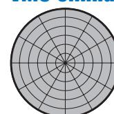
The omni capsule is perfect when the talent may need to be off-axis, such as in an interview situation. Also, omni capsules by nature are much more immune to handling, popping and wind noise than directional microphones. In addition, this capsule has slightly higher sensitivity than the VMC cardioid capsule.
