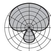
In applications where maximum gain before feedback is required, the VMS capsule is the right choice. With its nearly perfect super-cardioid pattern, the AKG C5900 capsule rejects sounds from the rear and rear sides, while providing a generous frontal "live" area. The VMS is slightly lower in sensitivity when compared to the VMC.
