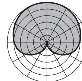
This element has excellent frequency and transient response rivaling the top condenser performance microphones on the market. The pickup pattern is a standard cardioid with exemplary off-axis response, allowing the talent to move around the microphone without a change in tone. The extended high-frequency response produces an open, clean sound with excellent intelligibility.
